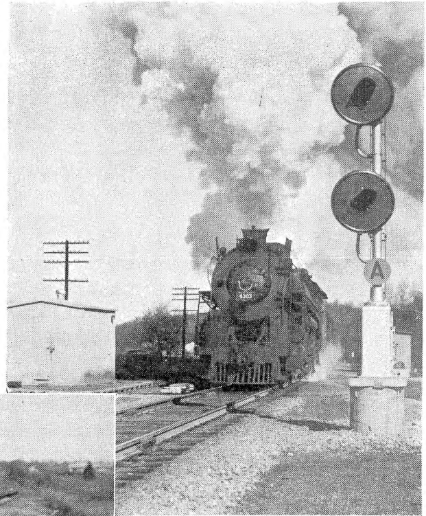
Above—Eastbound freight train passing typical westward semi-automatic signal. Left—The power switch layouts include insulated gage plates and rail braces
