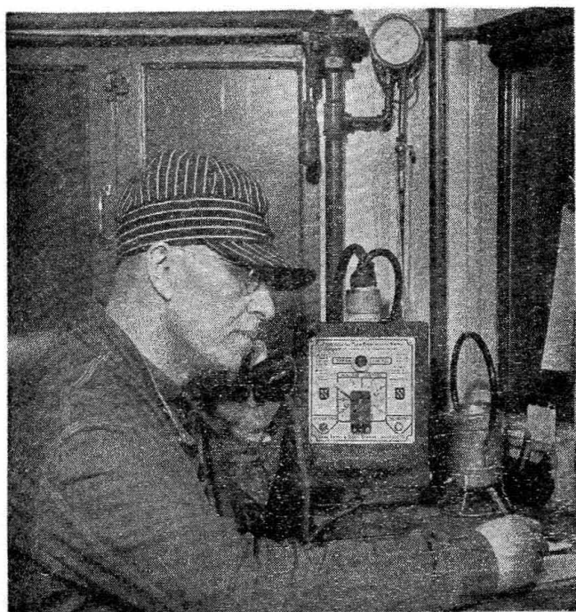
Conductor in caboose using the train communication apparatus to talk to engineman
