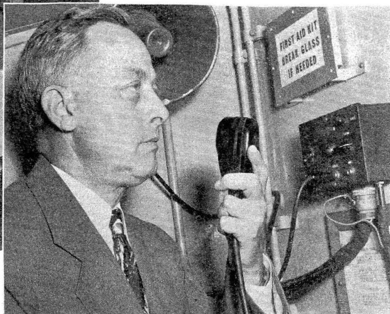
Above—Conductor in caboose using the train telephone to talk to engineman in the cab Right—L. L. White, vice-president-operations, using telephone in a Diesel locomotive
