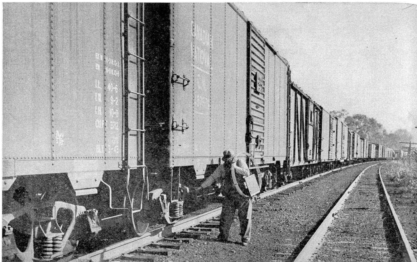
A Pennsylvania freight conductor uses the new Carryphone portable telephone to keep in touch with his engineman while making a routine inspection of his train. The Carryphone operates in conjunction with the inductive train telephone system installed by the Pennsylvania on 1,056 miles of main tracks between Harrisburg and Pittsburgh, and on the Belvidere-Delaware branch in Northern New Jersey
