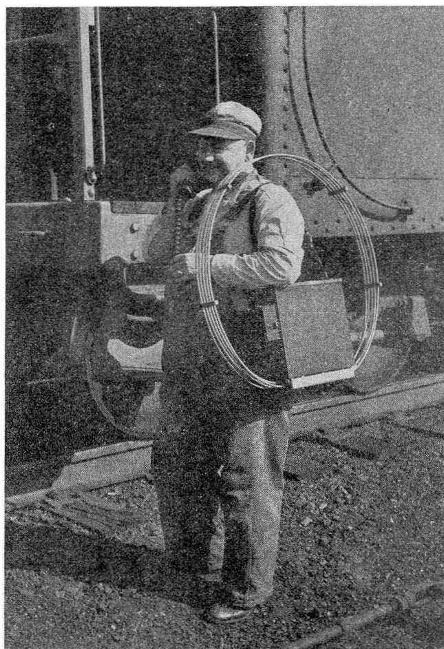
Left—The Carryphone in place in a Pennsylvania cabin car. When resting in the special receptacle prepared for it, its tiny storage batteries are automatically connected with the larger batteries of the cabin car train telephone unit, and are kept fully charged. Lifted out of the receptacles, it is ready for independent use. Right—The new Carryphone, weighing about 29 lb., has a range of up to three miles when used to communicate with another Carryphone or with a train equipped with the train telephone, and of up to 15 miles when used call to a wayside control tower. The loop, consisting of five turns of \frac{1}{4} -in. metal, is 30 in. in diameter and provides means by which messages are received and transmitted by induction, using the track and wayside pole lines as channels
