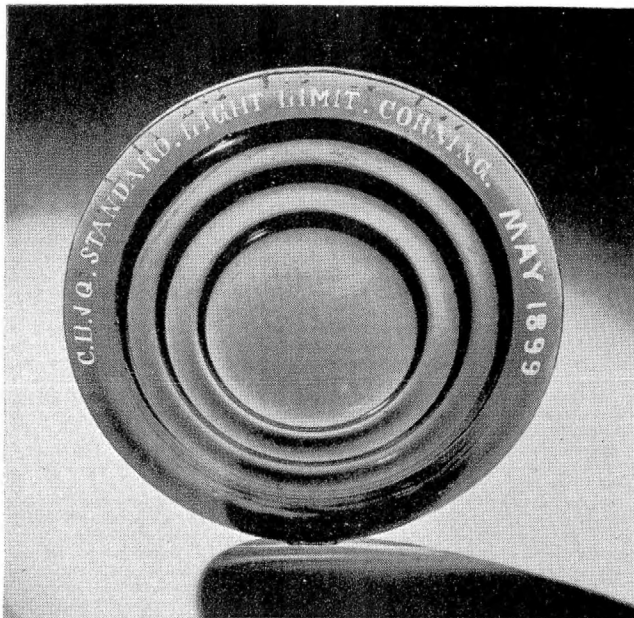
The Chicago, Burlington & Quincy standard red lens of 1899 made by the flash method
