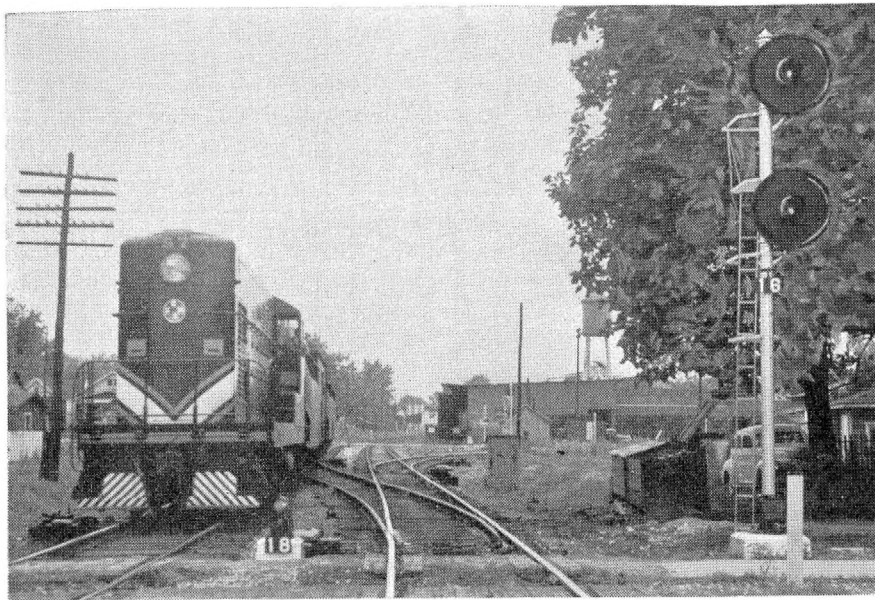
Southward home signals 16 and 18 at Virginia Avenue, showing Diesel-electric switcher at work on the northbound main track
