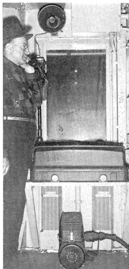
Right—Radio on a line car. The loudspeaker above the window, control at left, transmitter and receiver in case below window, and the dynamotor on the floor
