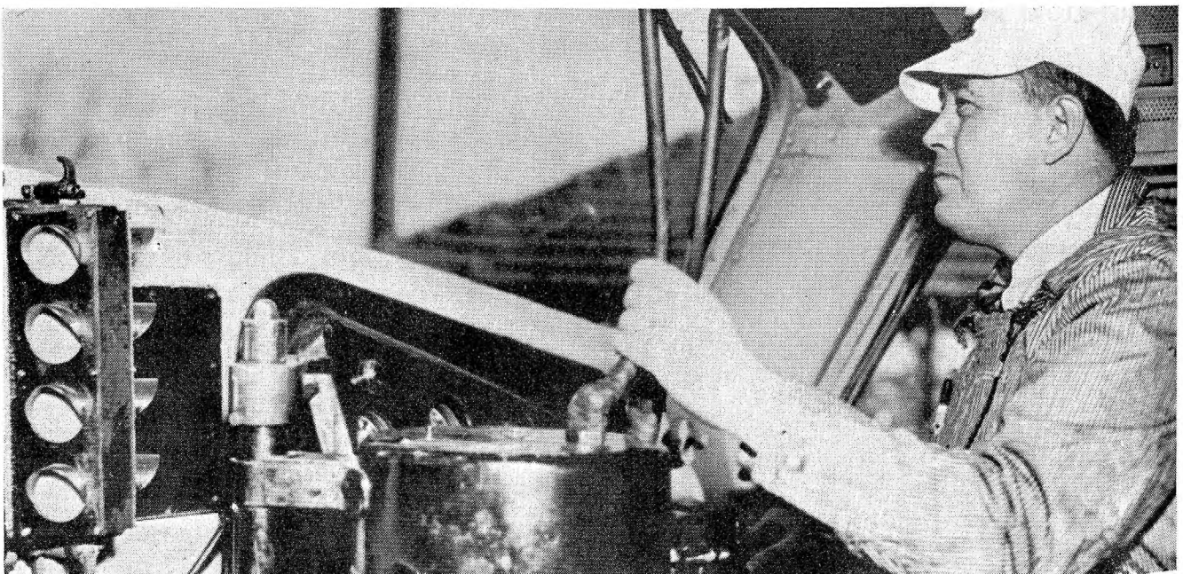
The cab signal in each Diesel-electric locomotive displays aspects faced to the engineman and also to the fireman's side of the cab
