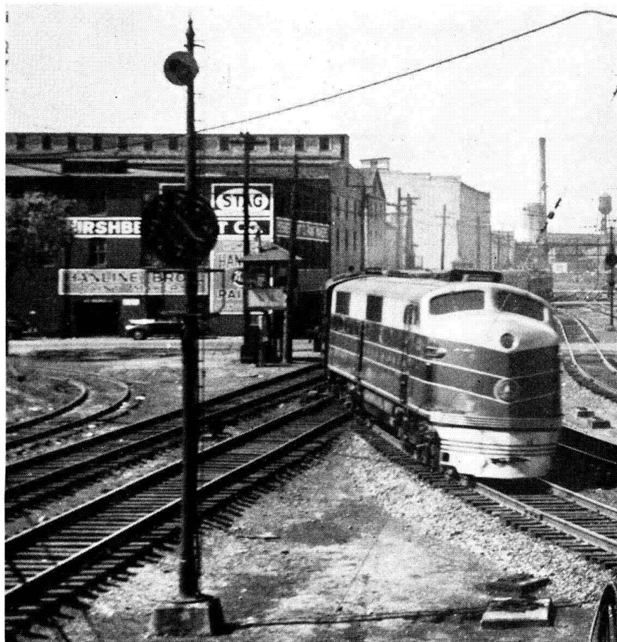
Eastbound passenger train crossing over movable-point-frog No. 24A at "BY".
