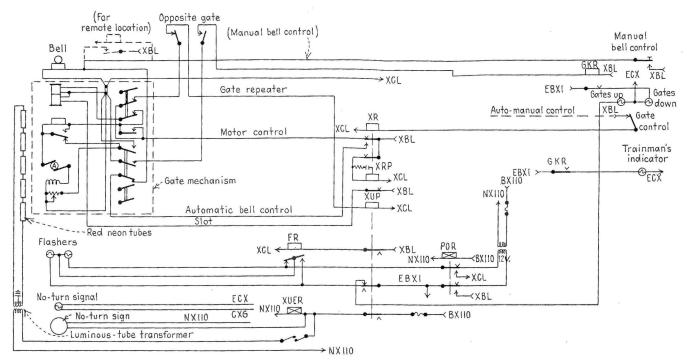
Typical neon-lighting and crossing-protection circuits
