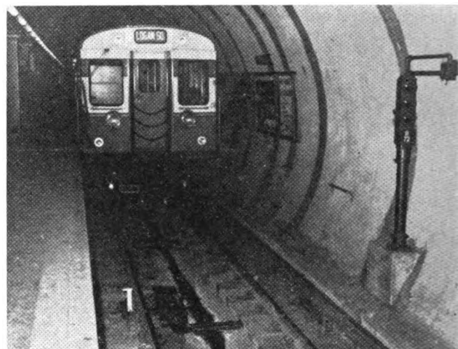
Rear view of a train standing in the station with the signal showing a red aspect and the train-stop trip in the raised position
