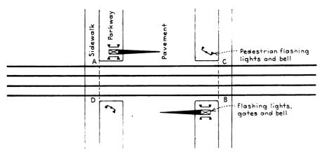
Fig. 2-Plan showing pedestrian signals
