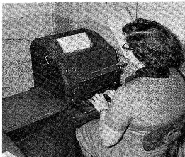
A clerk in the yard office Teletypes a switch list which is simultaneously reproduced on Teletype printers in yard and hump offices and elsewhere
