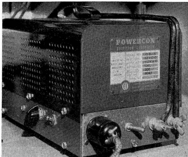
Vibrator converter for 110-volt standby
