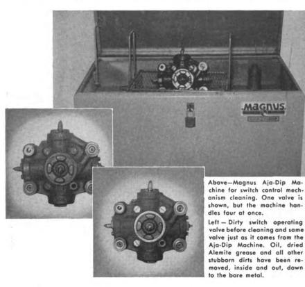
A bout 500 electric-pneumatic control switches are now cleaned better, faster and at lower cost by a Magnus Method.
