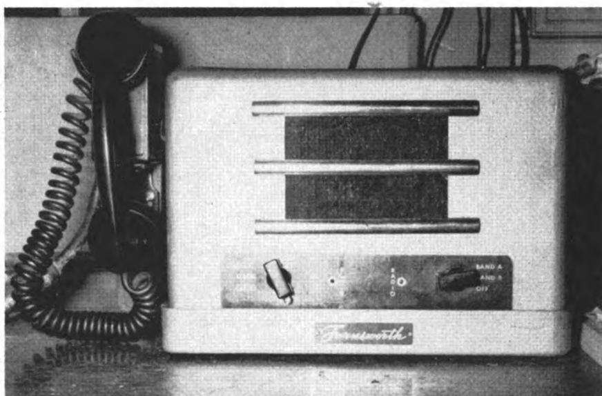
Remote control radio set in yard office enables clerk to talk to car checker
