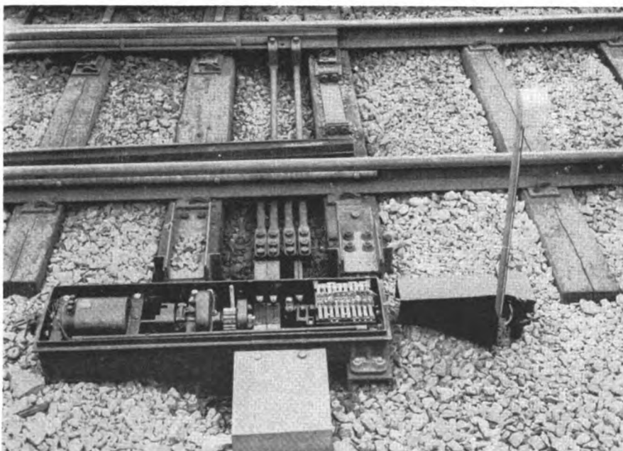
Switch machine with cover open to show mechanism
