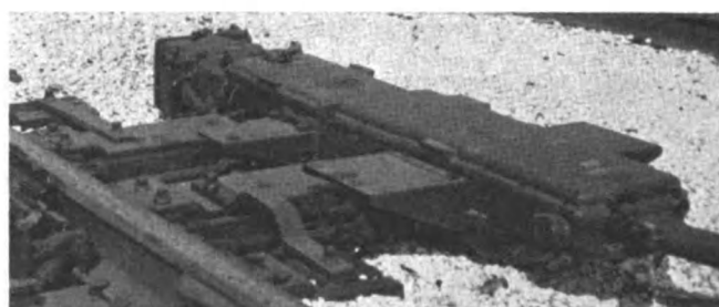
Switch machines are equipped with an outboard brake
