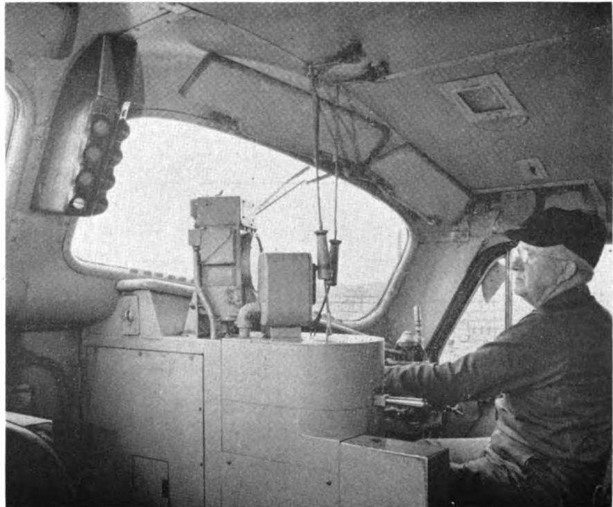
Cab signal unit is centrally mounted, visible to enginemen and firemen
