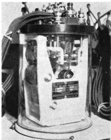
Code transmitter for 180 code
