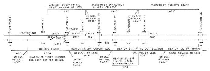
ing bell is attached to one of the signals at each crossing. The protection is automatically operated, on the approach of trains, by track circuits.
