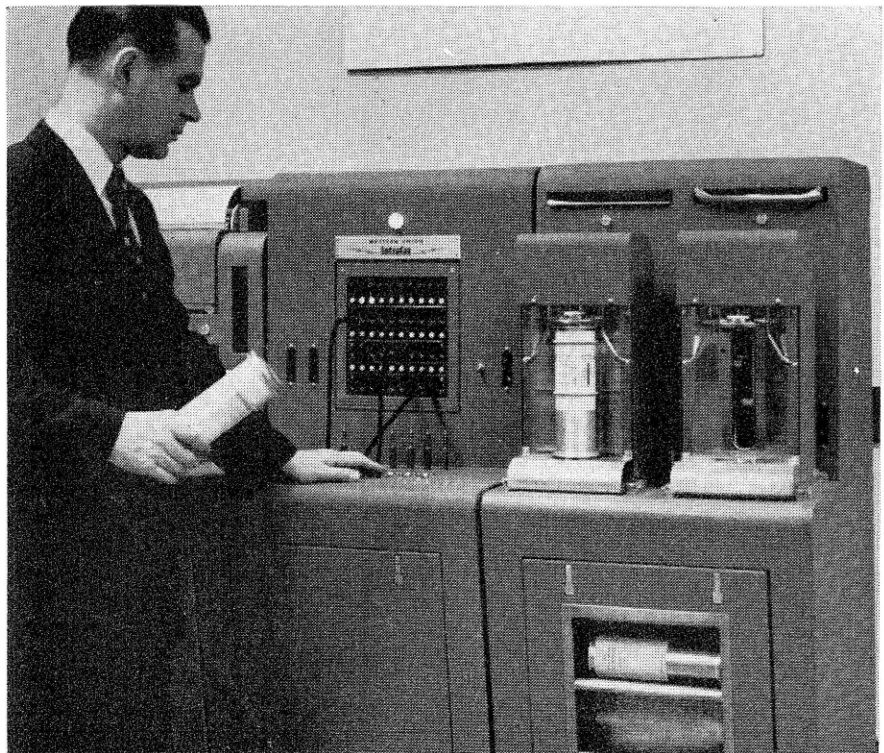
Facsimile equipment in Penn Station: switchboard in center; incoming messages received at left; outgoing reservations or messages sent by scanner at the right
