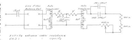
(1) The .5MF condenser balances the ET and ER one microfarad condensers located on the line side of the hybrid.
