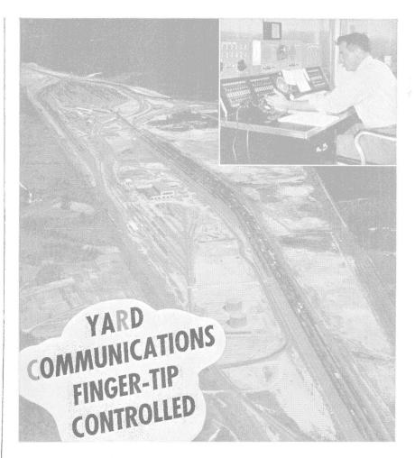
HE communications nerve center of the splendid Ernest Norris Yard of the Southern Railway System is North Relay equipment engineered in collaboration by Southern Railway engineers and those of North. This automatic system provides the tower man with finger-tip control of a network of speakers, "talk-back" units and telephones directing the inspection, sorting and humping of up to 2,500 cars into 56 classifications.
