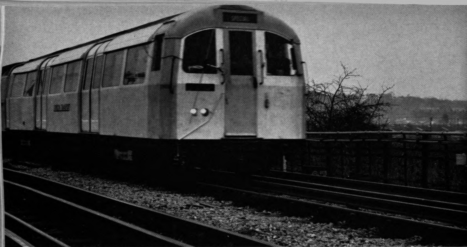
Train equipped for automatic operation is approaching a "command spot" (wayside equipment at right) on a test run between
