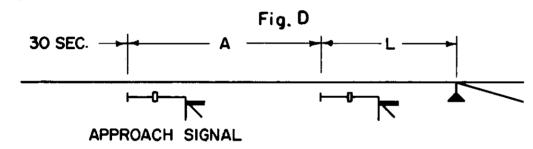
(1) WHERE "L"IS LESS THAN MAXIMUM SPEED BRAKING DISTANCE BUT MORE THAN 15 MPH BRAKING DISTANCE (700').
