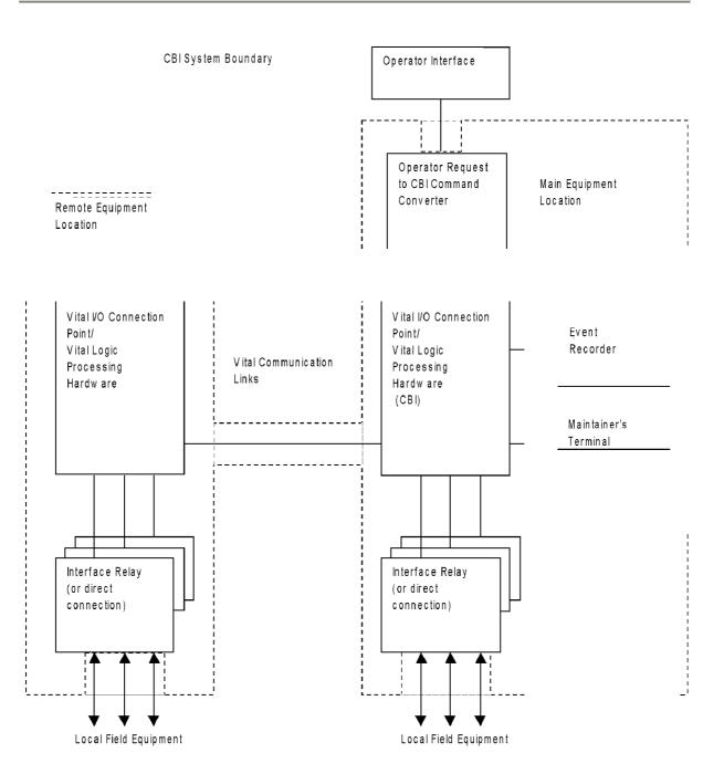
The Operator Interface boundary is defined as the physical connection point available to the operator interface to directly communicate to the CBI equipment without further protocol conversion.
